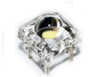
Figura 3 – Superflux LED ultra bright – white.
